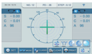
Flexible handling of single vision, bifocal, and progressive lenses, and measurement of progressive multifocal lens (PPL) power
